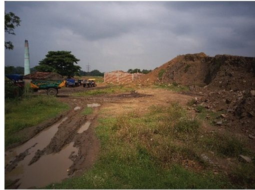
Fig. 6: Brick kiln developed adjacent to the Damagaria opencast mines to use the topsoil extracted from the mine.
