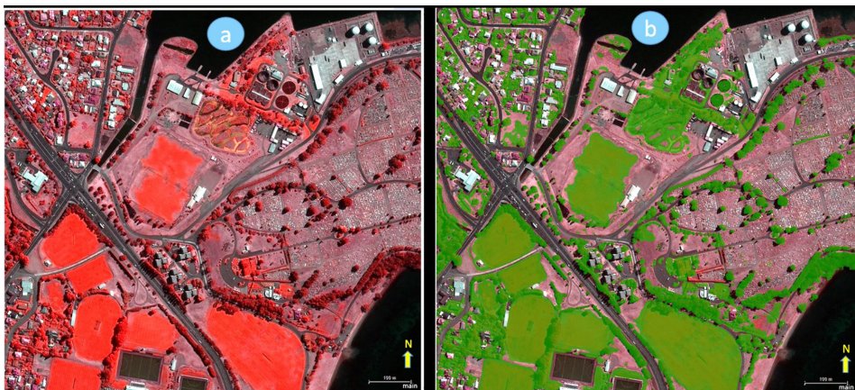
Fig. 5: Classification result of Ikonos data: a) Unclassified false colour composite image b) classified image showing green space
